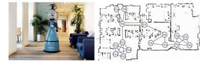
Figure 1: The mobile service robot we aim to use for the demo, deployed in an office scenario (left) and a topological map (right). Edges in blue represent the default laser based navigation, the edge in green represents a specialised ramp traversal behaviour, and the edge in red represents a specialised door crossing behaviour.
